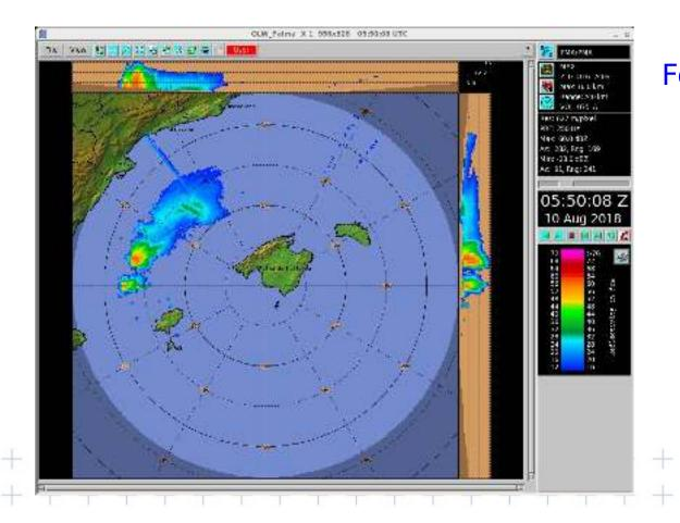
Following Marshall-Palmer Relationship (Z=200\*R^1.6) we have maximum values of 3 hour accumulated precipitation around 150 mm (50-60 dBz)
