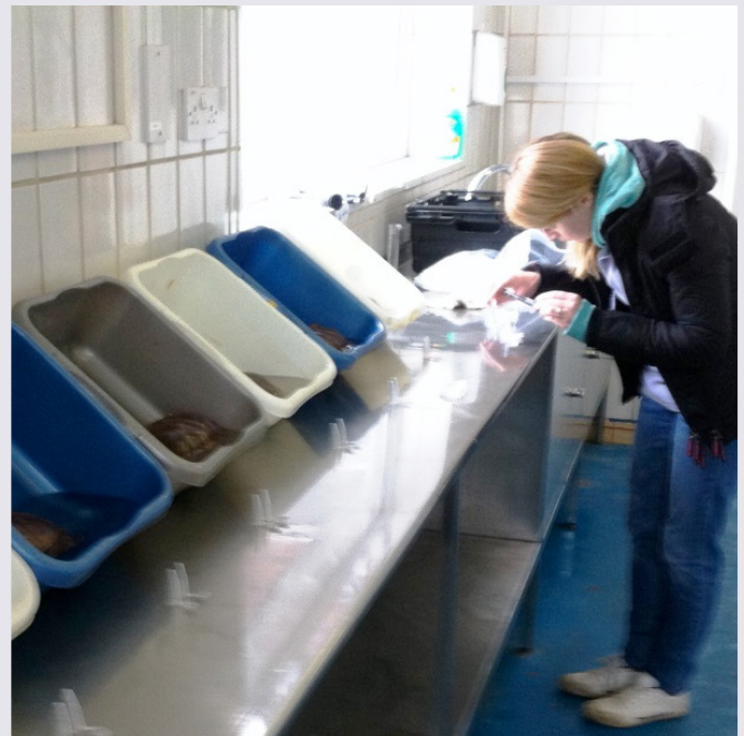
Fig. 5 Taking samples for ammonia production in simulated vivier transport, 1:1 crab:water.
