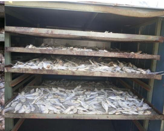
Drying of ready to fry spiced Anchovy in Solar-Biomass Hybrid Dryer
