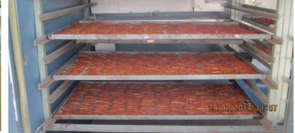
Drying of ready to fry spiced Anchovy in Solar-Biomass Hybrid Dryer
