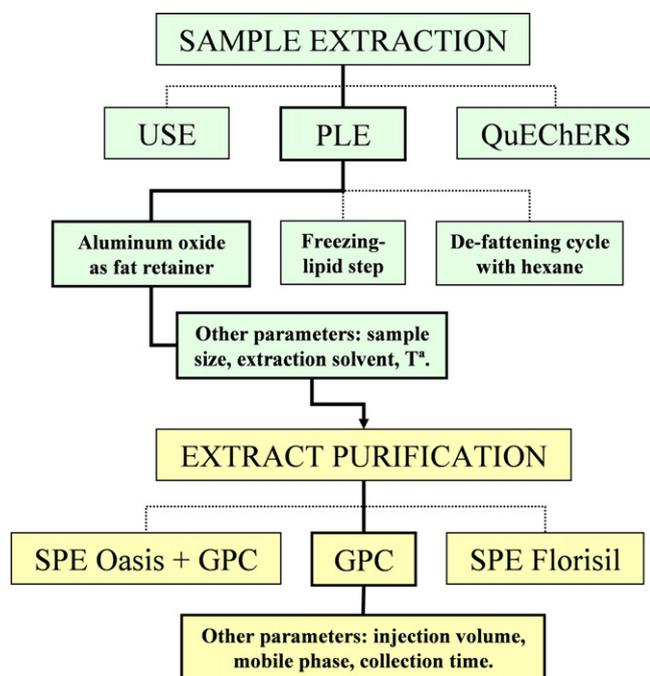
Fig. 1. Sample pretreatment scheme tested during method optimization.
