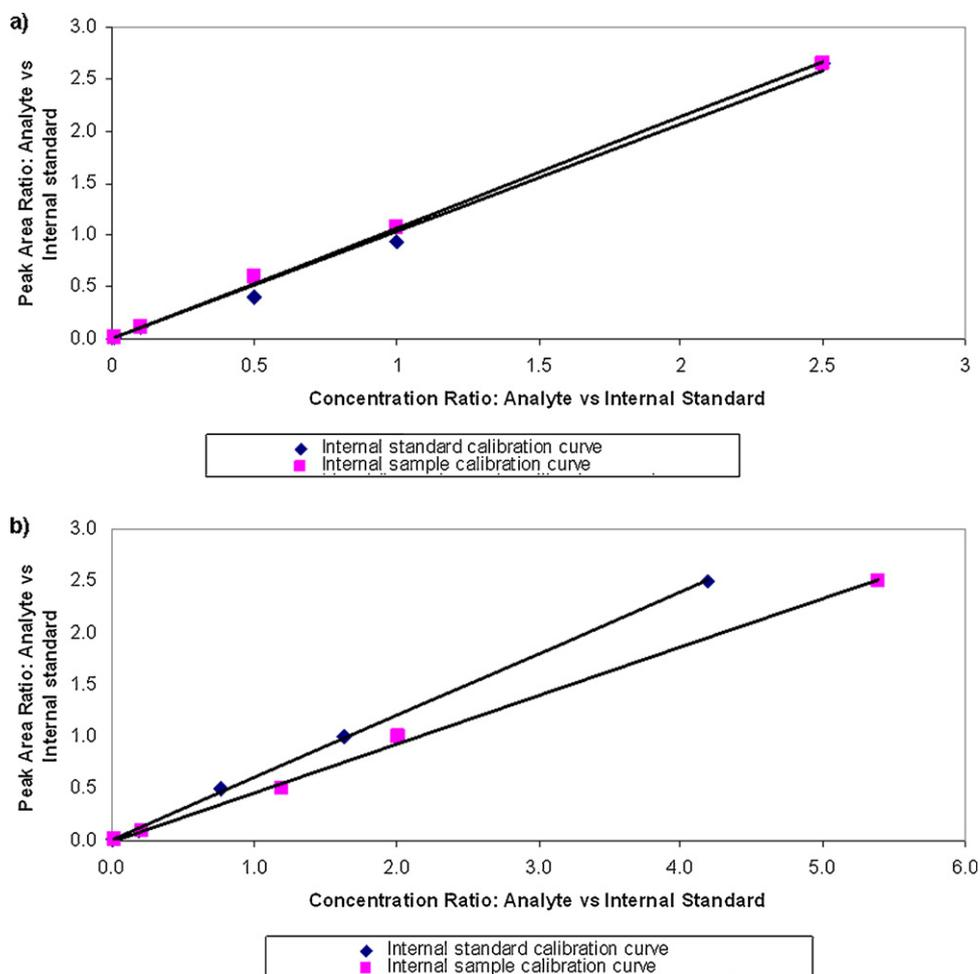
**Fig. 5.** Comparison between calibration curves in the solvent, and in real sample with internal standard for the pharmaceuticals (a) carbamazepine (carbamazepine- $d_{10}$  as internal standard) and (b) clopidogrel (diazepam- $d_5$  as internal standard). Calibration curves were prepared in *C. carpio* extracts.
