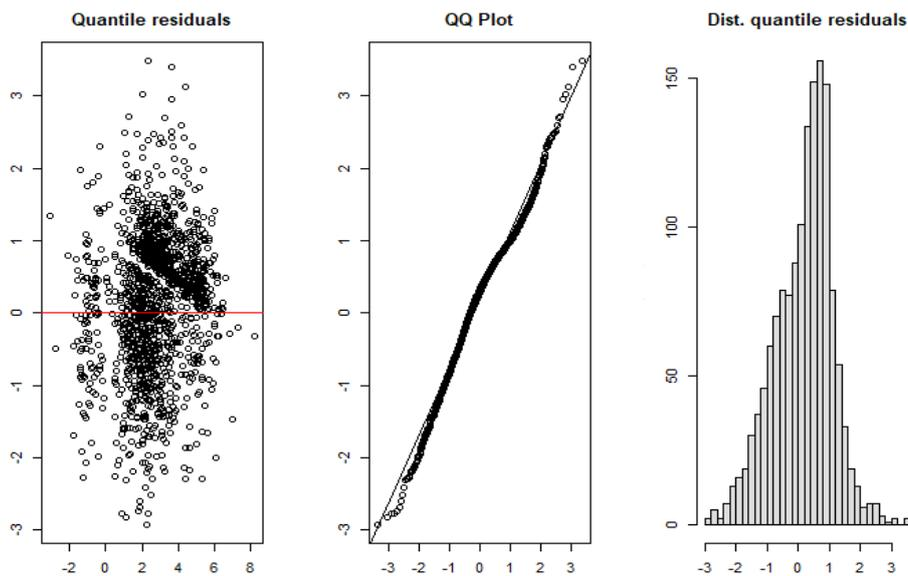
**Figure 5.15.** Scatterplot of the residuals vs. fitted values (left panel); normal probability plot of residuals (middle panel); distribution of the quantile residuals (right panel) obtained in Model 8.
