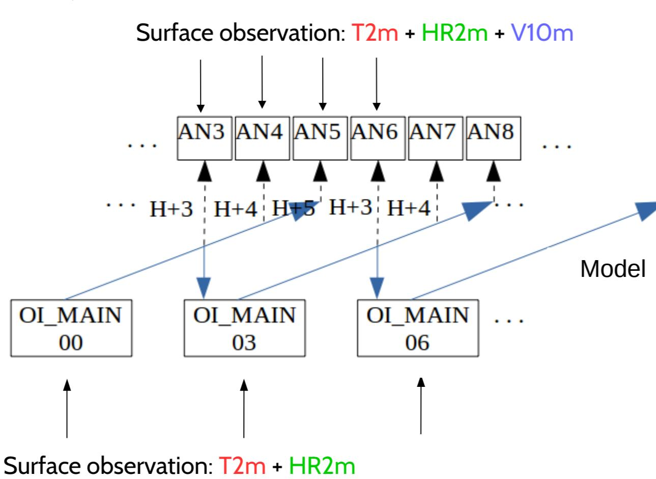
Figure 1: Scheme of the local OI\_MAIN sequential surface DA (Giard & Bazile, 2000) + OI hourly analysis (Taillefleur, 2002).
