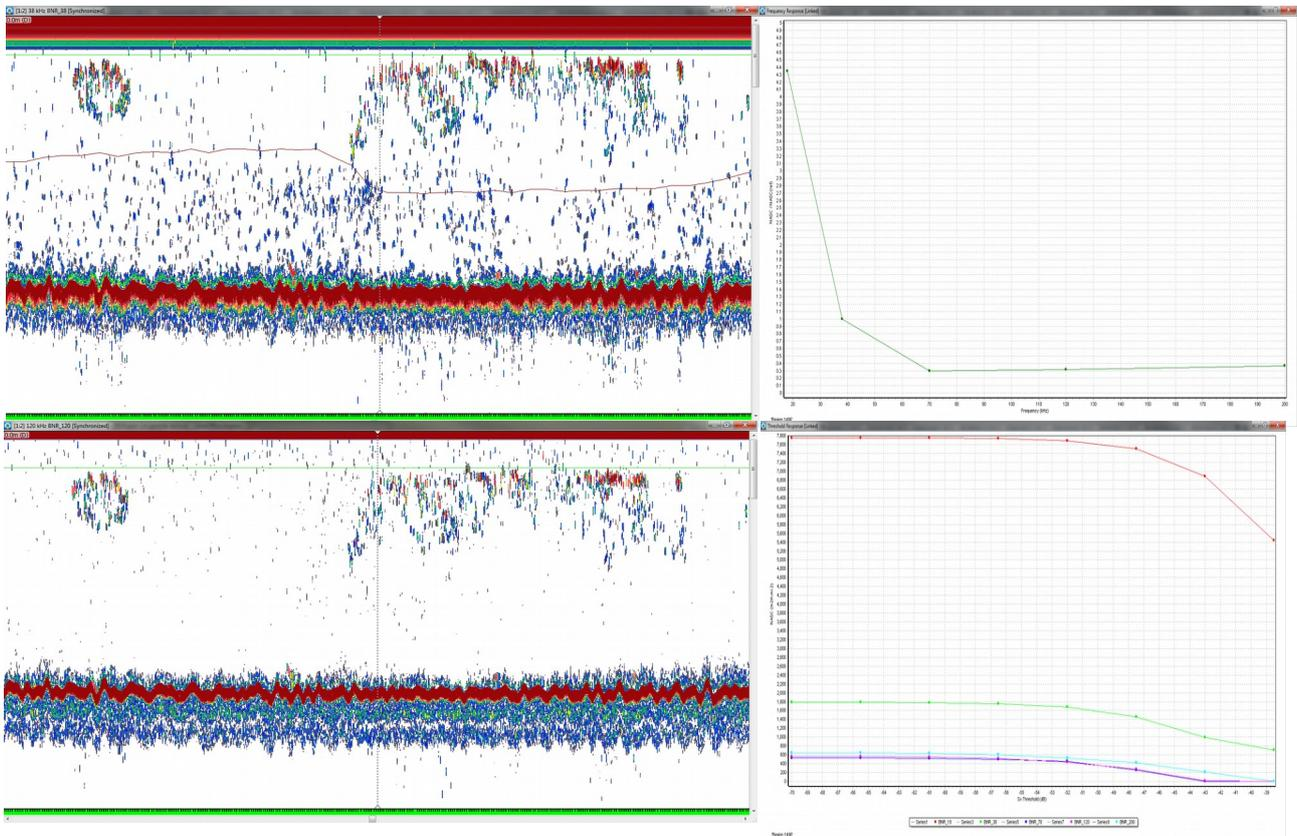
Figure 10. Echogram showing echotraces attributed to chub mackerel (38 kHz above, 120 kHz below) and its characteristic frequency and threshold responses (ground truthed by fishing station)
