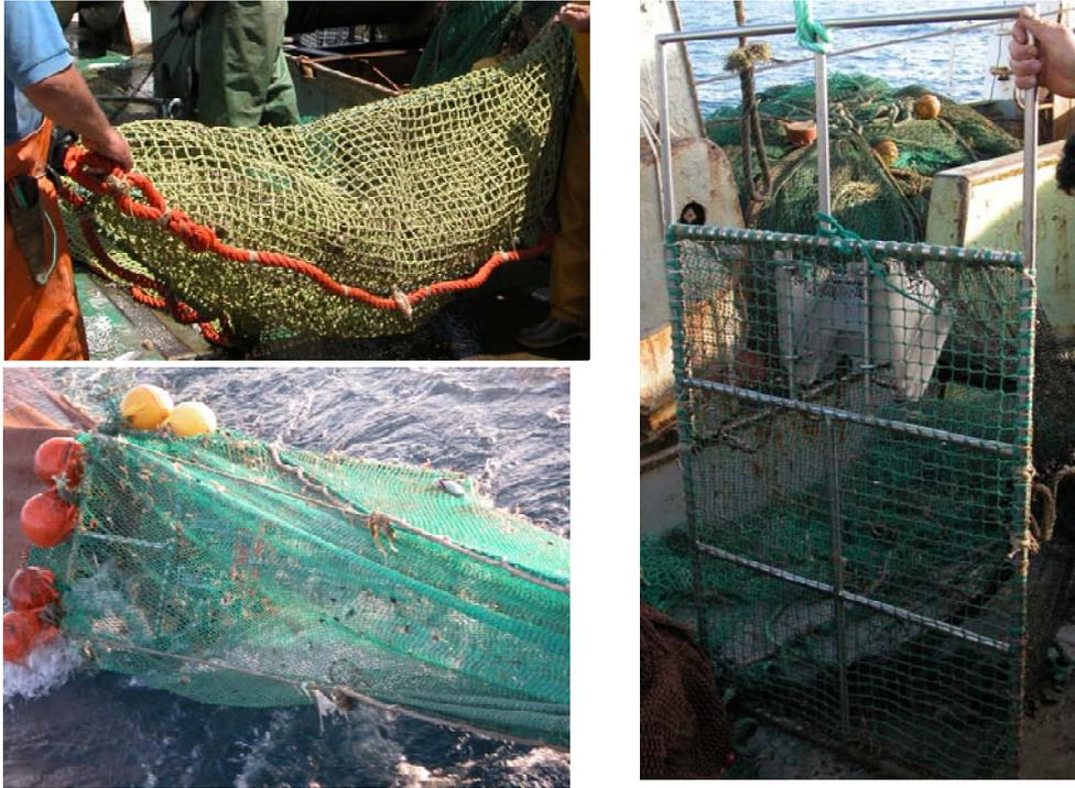
**Figure 2 – Examples of a square mesh size configuration and sorting grid.**
