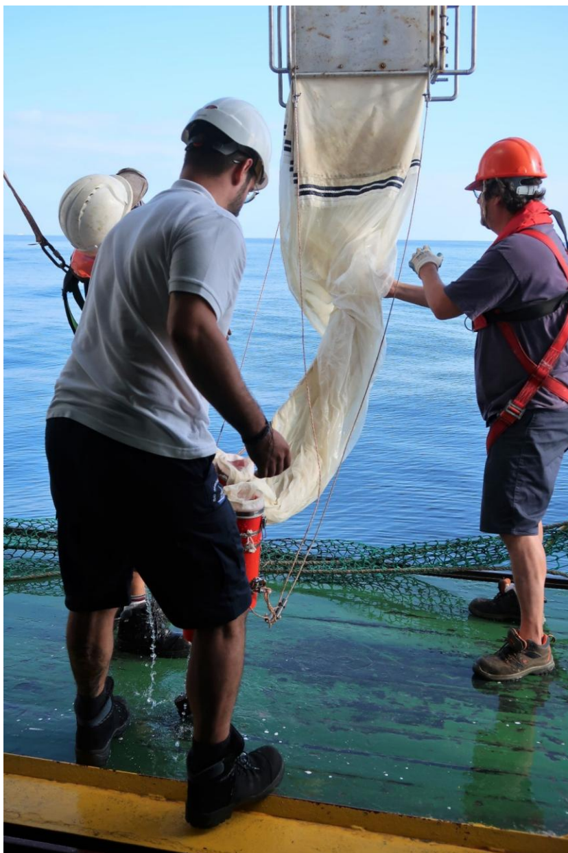
Fig. 4: Recovery of the plankton net after a vertical trawl along the 700 m of the water column depth
