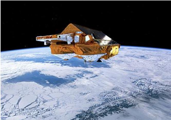
CryoSat-2 (ESA's ice mission) measures the thickness of polar sea ice and monitors ice-sheet changes in Greenland and Antarctica (launched in 2010)
